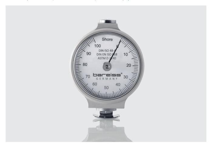
The hardness tester is used to determine the Shore hardness of soft elastic materials, elastomers and plastics. For a reliable hardness test according to the standard, a smooth and flat specimen with  $\geq$  35 mm diameter and  $\geq$  6 mm material thickness is required.
