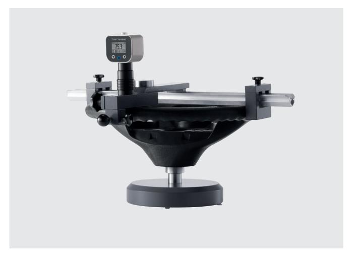
To determine the hardness of foamed materials used in the steering wheels of motor vehicles, with plastic or leather covers, we recommend using our HPE III L. With its short measuring path and the small 5 mm indentation ball, this digital handheld hardness tester was especially designed for materials with thin layers.
