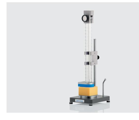
The elasticity of polymeric foam materials can be analyzed by measuring the rebound height of a ball after the free fall and impact on a test specimen.
