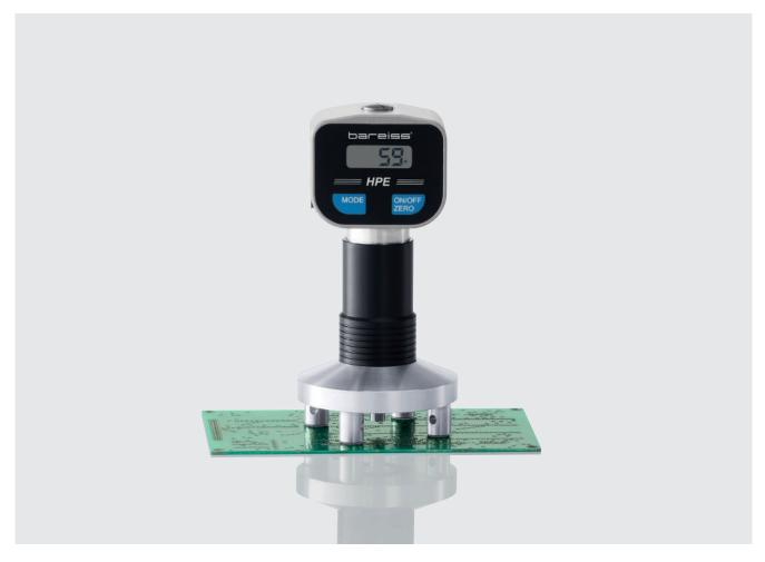
The hardness testing of solid materials such as glass fiber reinforced plastics, thermosetting plastics, hard thermoplastics and light metals can be reliably undertaken with our digital Barcol handheld hardness tester. For correct measuring results, the test specimens should have a flat surface and a minimum thickness of 1.5 mm.
