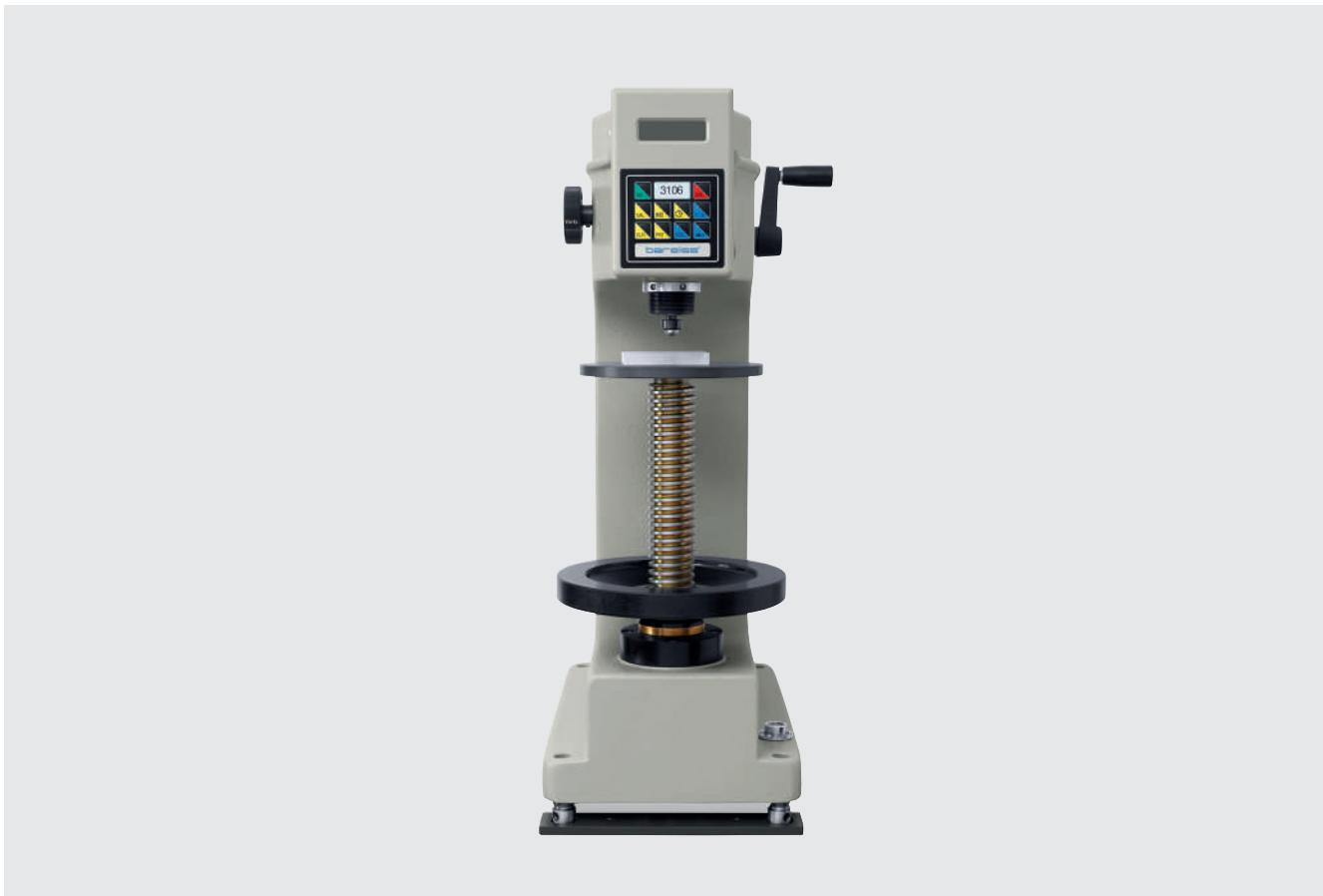
The 3106 testing device has a very variable use, being suitable for the determination of ball indentation or Rockwell hardness on different materials. According to the previously-installed module, the 3106 calculates the hardness of metals, carbon materials, plastics, plaster, gypsum, floor coverings or asphalt, according to the corresponding standard.
