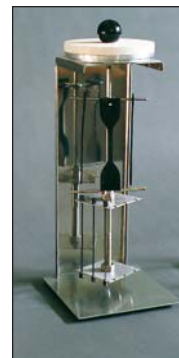
Stand EB 01.01 , stand to support the sample holder while mounting test pieces for ageing.
