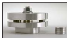
Compression Set Rig EV 03 , according to ISO 815.
