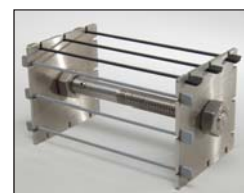
Tension Set Rig EV 04 , according to ISO 2285.
