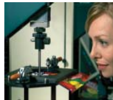
Fig 20. Testing the puncture and bursting strength of packaging material
