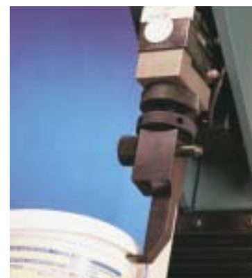
Fig 21. Determining the force to remove the lid from a plastic package
