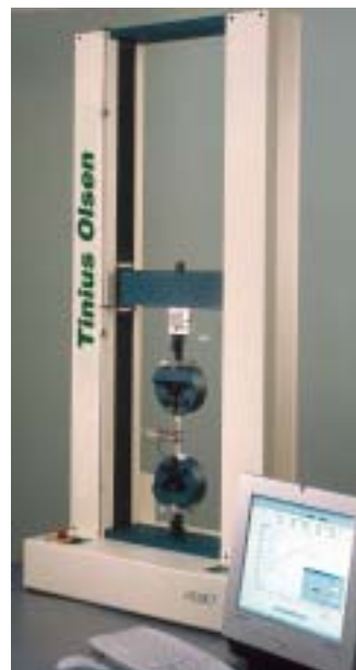
Fig 37. Model H50kT with HT21 grips
