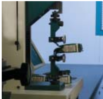
Fig 11. Testing the strength of coffee packaging using the quick release vise grips, HT55
