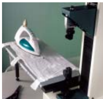
Fig 15. Testing the static and dynamic frictional forces to pull an iron across fabric
