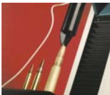
Fig 14. Testing the extraction force of a bullet from its cartridge using custom pneumatic grips
