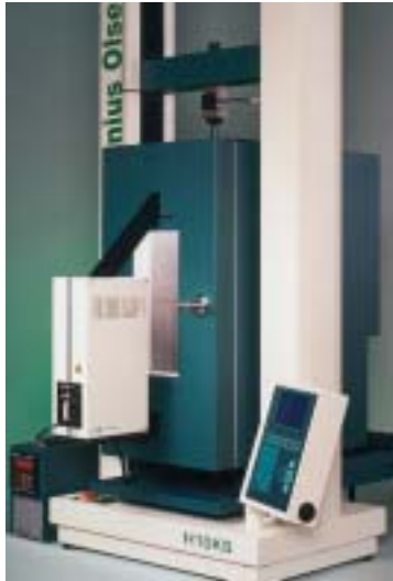
Fig 26. Model H10kS shown with an environmental chamber for testing at elevated or reduced temperatures; note the use of a laser extensometer that can be used with the chamber to determine the elongation of the sample
