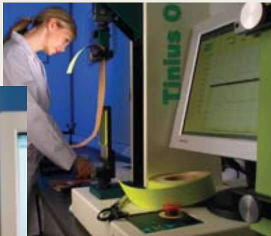
Fig 9. A model H5kT and a model H5kS being used to determine the bonding strength of adhesive tape
