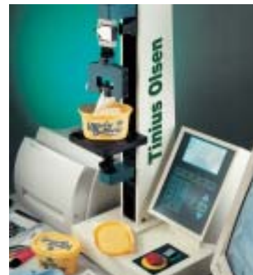
Fig 19. Testing the adhesive peeling forces of foil packaging
