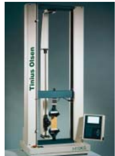
Fig 32. H10kS testing fabric with a high elongation extensometer
