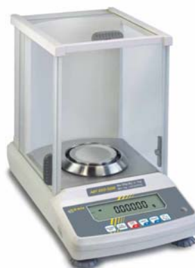
A suitable balance for gravimetric tests with 0,00001 g
