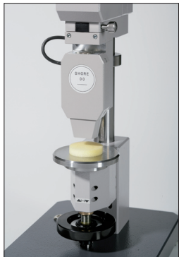
Shore OO/OOO VLRH for sponge and cellular rubber, foam rubber, silicone, similar to gel materials from a material thickness of 6 mm
