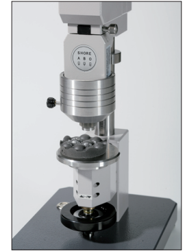
Shore A/B/O for concave and convex moulded parts of a material thickness of 4 or 6 mm
