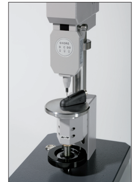
Shore D/C/DO for moulded parts of a material thick- ness of 4 or 6 mm
