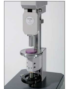
Shore A/D for flat plate materials of a material thickness of 4 or 6 mm
