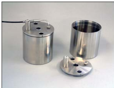
Containers for testing of Stress Relaxation in liquids
