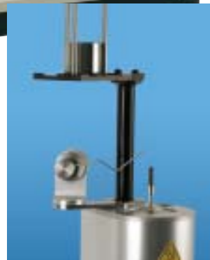
Fig 5. Automatic swing-away platform allows easy cleaning.
