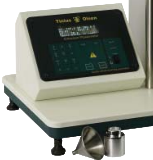
Fig 3. MP600 motorized weight with lowering and lifting device.
