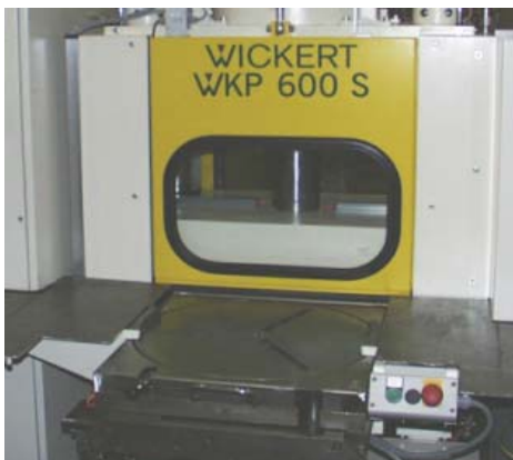
Swivelling table with ejector for the production of grinding wheels or similar
