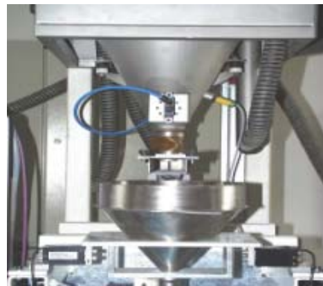
Gravimetric dosing of powder
