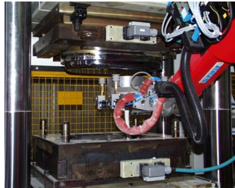
Robotloading, robot extraction
