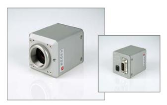
Argon SDC 212M cameras with auto iris control are fitted with 1/2" CCD sensors with a resolution of either 752 x 582 pixels (CCIR) or 768 x 494 pixels (EIA). As an option, the sensors are also available with enhanced sensitivity in the near-infrared (NIR) range of the spectrum. The Argon cameras provide a video composite interface.
