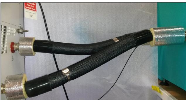
Tighten the hose connections gently and use two wrenches when tightening. One wrench to support the EB 17 oven piping and one wrench to turn/tighten the hose connector. This to avoid rotating the piping at the EB 17 oven.
