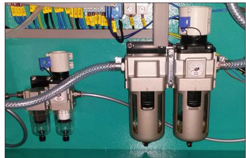
**Figure 2.4.b** – Inside the oven there is also are two set of pressure controllers. The low flow system pressure is set to 0,05 MPa. The high flow system pressure is set to 0,1 MPa.
