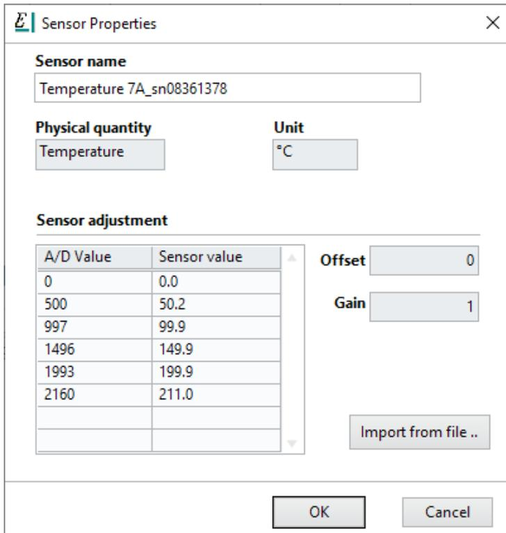
The new sensor from the manufacturer is normally delivered with a new sensor property file (\*.tvs file). By importing the new profile on top of the existing sensor, it is possible to continue the logging without losing valuable test time.
