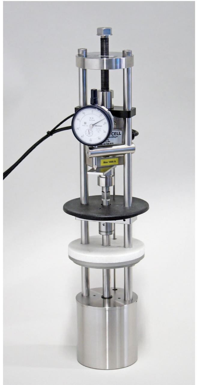
*Rig for testing in liquids.*
