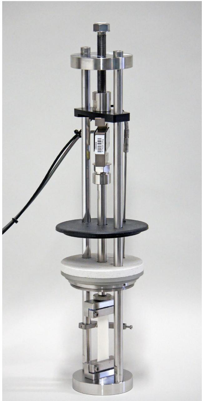
*Rig for testing in tension.*
