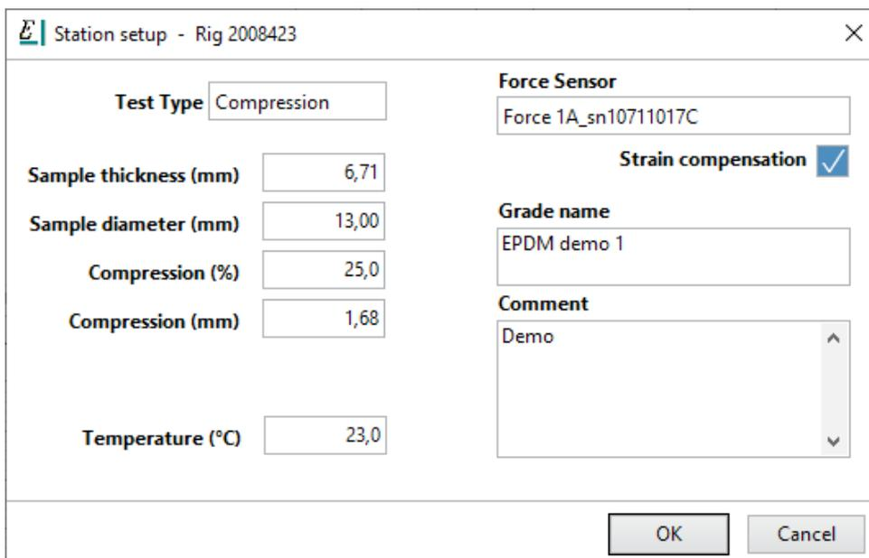
2. Select *Test Type* tension or compression.
