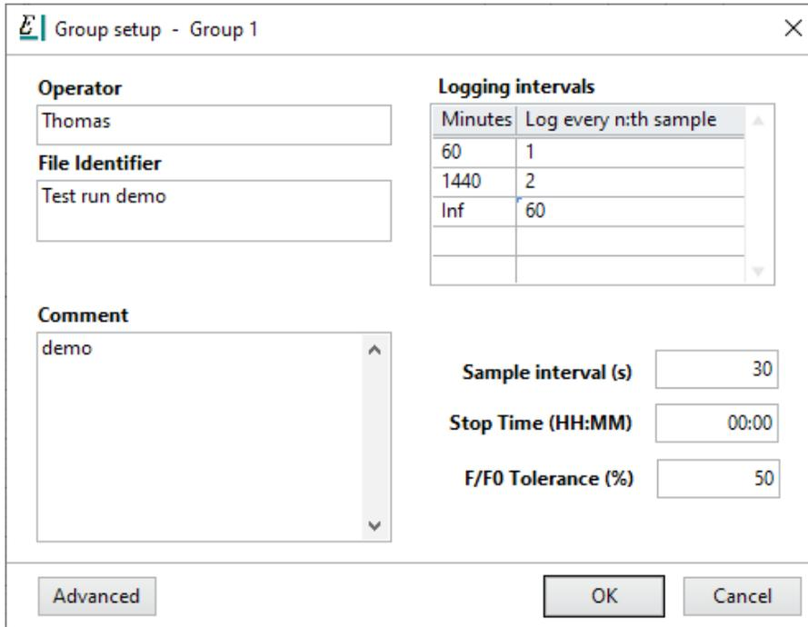
Group setup window displaying recommended logging intervals and sample interval.
