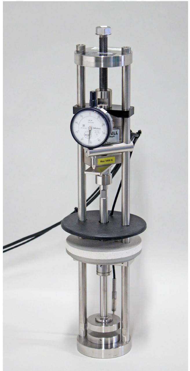
*Rig for testing in compression.*
