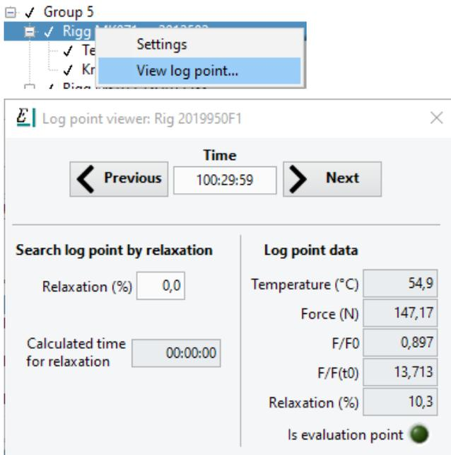
To quickly scroll through log points, select either the seconds part of *Time* (e.g. by clicking on the seconds part) or select all figures in *Time* (e.g. by double-clicking on the time data) and scroll using the mouse wheel, which will step through log points.
