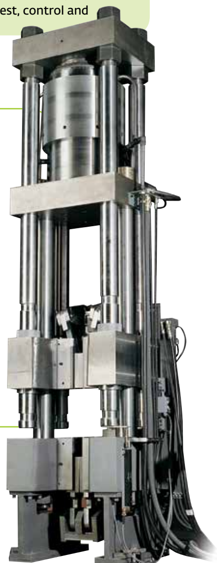
3000SL with upper hydraulic piston configuration. www.tiniusolsen.com
