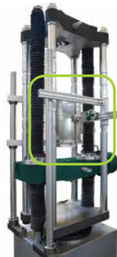
Typical 600 kN (120,000lbf) SL with closed crossheads, rack and pinion grips and a furnace.
