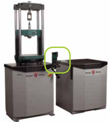
Typical 150kN (30,000lbf) SL with handheld controller.
